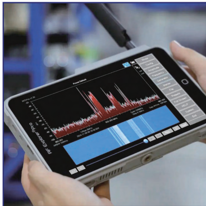
RF Explorer®Pro Touch Screen Spectrum Analyzer
